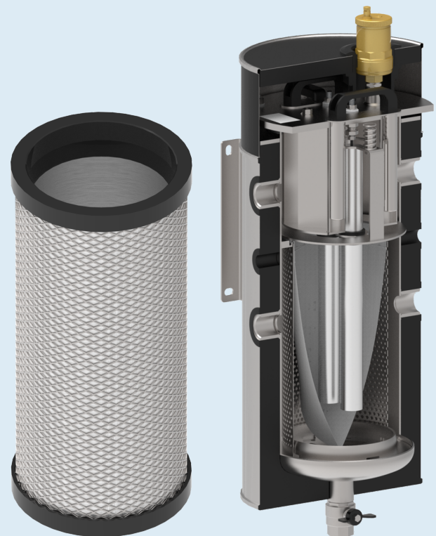
Cross-section showing upper chamber with magnets, before descending into the actual particle filter and anode chamber.
